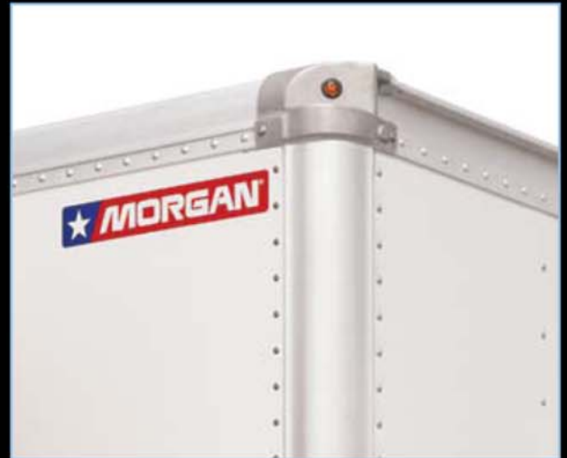
"R2" Corner Radius & Front-End Design, shown with optional LED lights.
