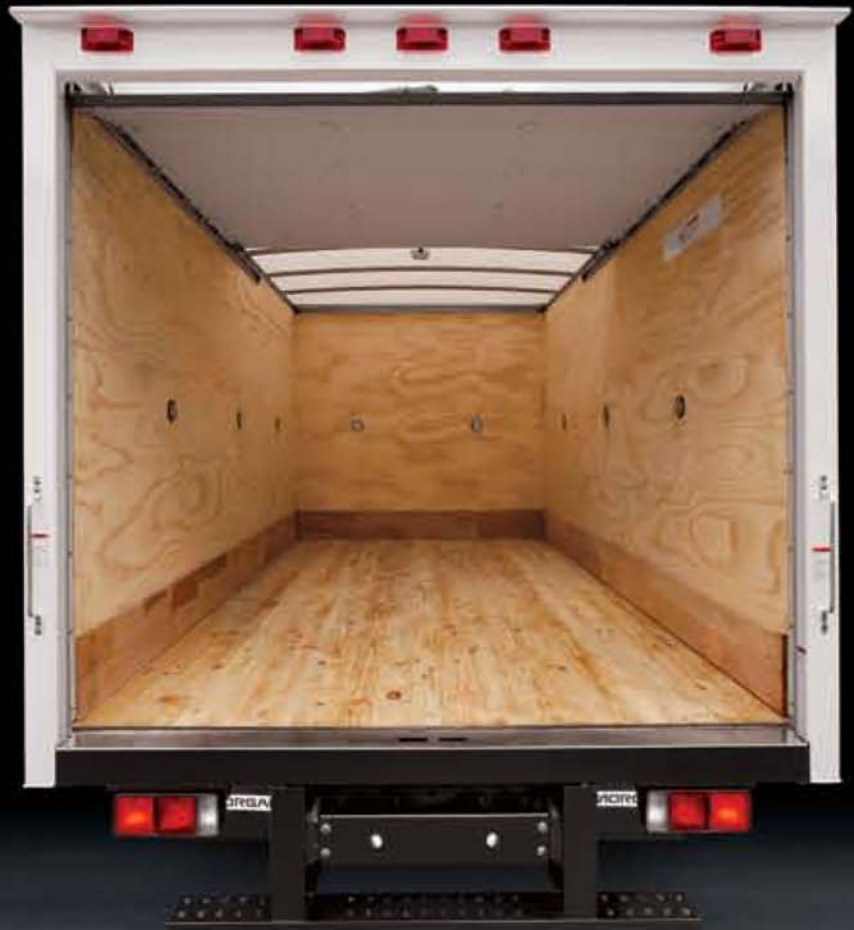
Cargo Area - Plywood liner, apitong scuff & tie rings
