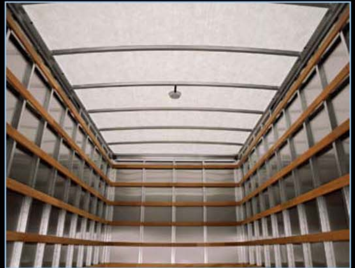
Translucent roof - allows natural lighting to brighten cargo area.
